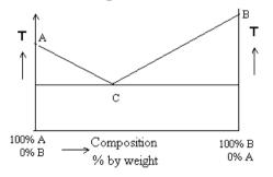
Phase diagram is a map or a graph of temperature versus composition of one of the constituent metals. As the composition of one metal increases, the composition of the second metal decreases and hence the extreme ends of the x - axis represented by the two ordinates indicate 100% of metal A and 100% of metal B.
