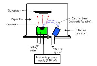
The electron beam generated by and electron gun is accelerated towards an anode by a high potential difference [kilovolts]. The crucible acts as anode or a perforated disc near the crucible act as the anode. A magnetic field is often applied to bend the electron trajectory so that the electron gun can be positioned below the evaporation line.
